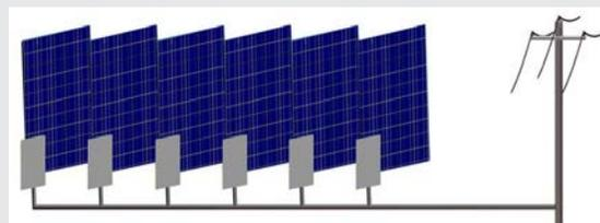
**Microinverters** are typically more expensive options than string inverters but have become more popular in recent years because they avoid the shared reduction in output that String Inverters can create. Microinverters are module-level electronics. They are basically working on the panel level versus a string of panels. Because of that, if there is a problem with one panel, only that one panel is impacted versus multiple panels connected in a string.
